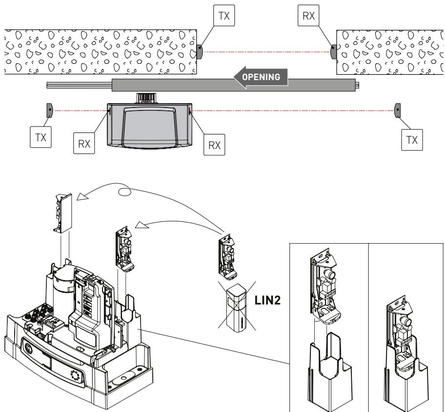
It is possible to install additional photocells inside the Ditec casing NeoS Green, for the protection of both the closing and opening movement, using the LIN2 photocell.
