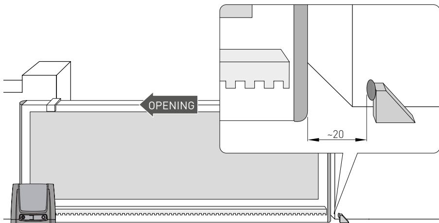
**i** The limit switch kit is optional and is used to stop the gate before it reaches the opening and closing mechanical stops. With a limit switch installed, slowdown is carried out at regulated power to overcome possible friction.
